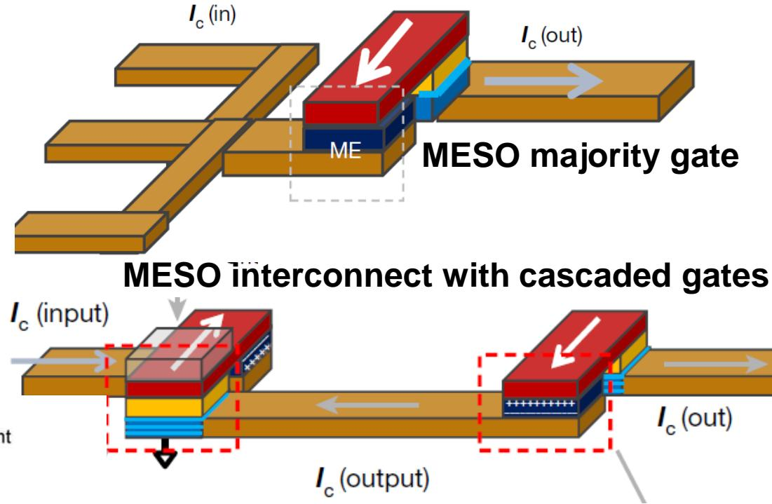
Magnetization to output voltage by spin to charge conversion via Spin-Orbit (inverse SHE or inverse Edelstein)
