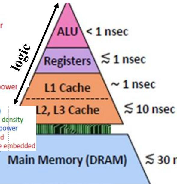
**RAM: High speed ( $\approx$  nanosecond for S-RAM) but volatile (electrical energy to maintain memory alive)**
