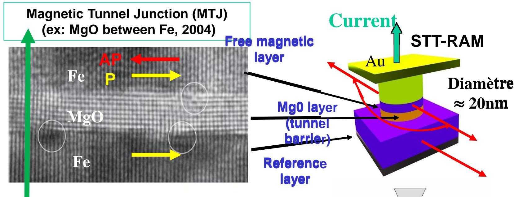
Writing by injection of magnetization from a spin-polarized current and STT
