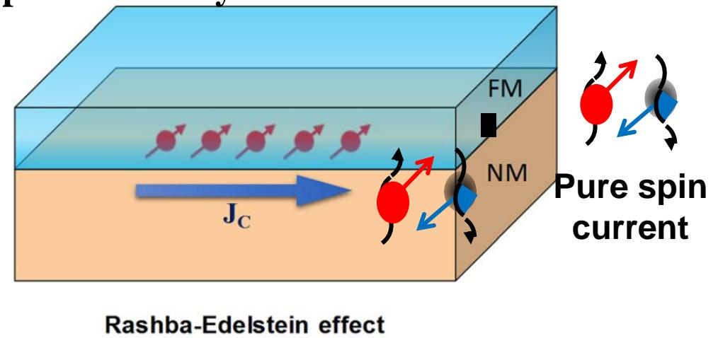
Inverse Rashba-Edelstein effect: injected spin current generates charge current ( conversion from spin to charge current)
