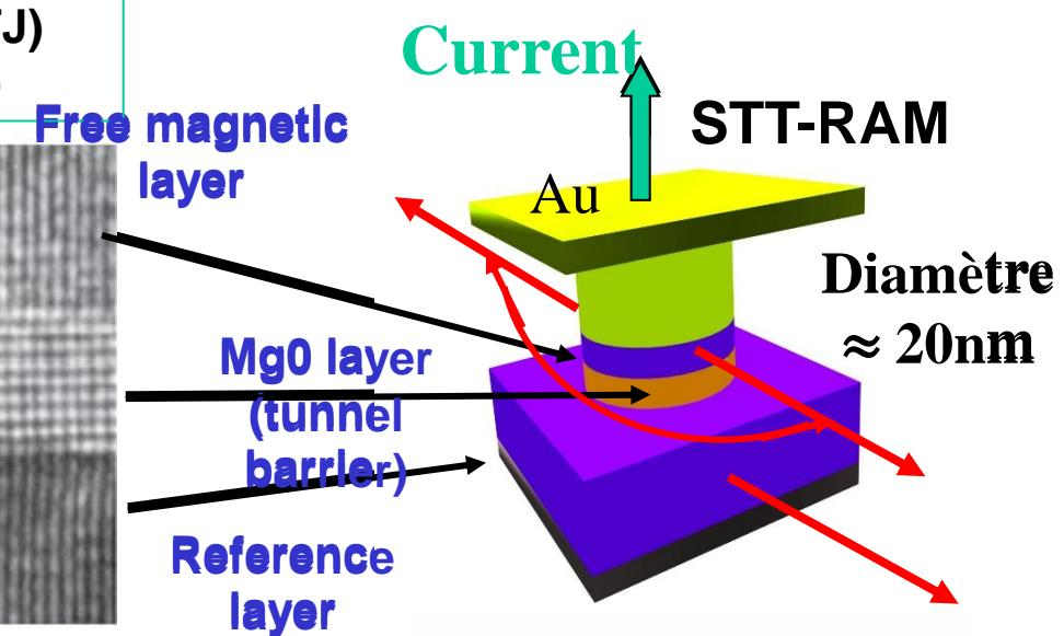
Writing by injection of magnetization from a spin-polarized current and STT
