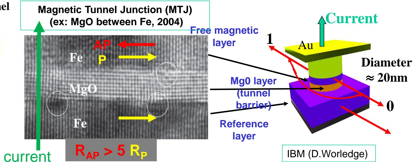
Reading by Tunnel Magnetoresistance ( $R_{AP} > R_P$ )
