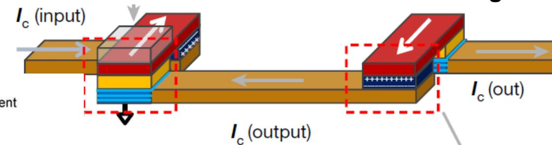
Magnetization to output voltage by spin to charge conversion via Spin-Orbit (inverse SHE or inverse Edelstein)
